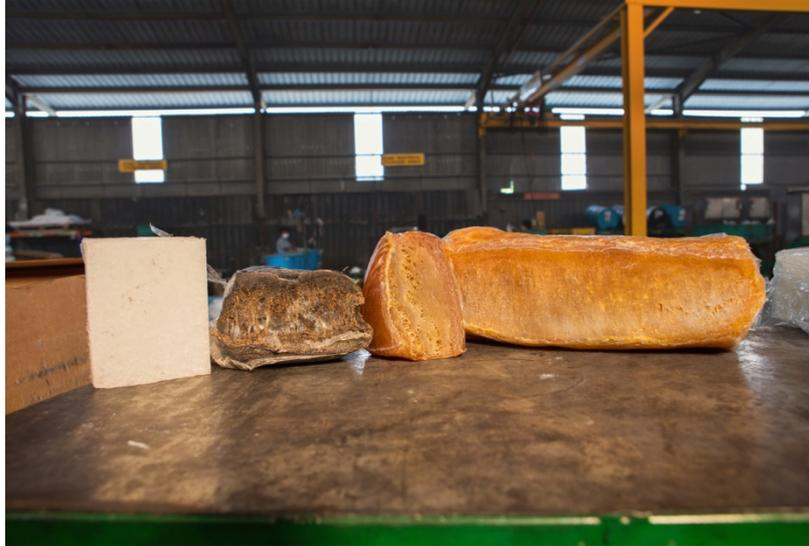
**Figure 1** Raw rubber material
