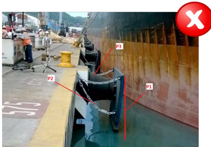
**Figure 3** Unfavorable panel position (P1), chains with incorrect angle (P2) and low rubber quality with incorrect design (P3)
